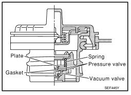
4. Check valve opening pressure and vacuum.
