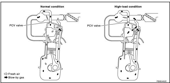
This system returns blow-by gas to the intake manifold.
