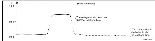
"HO2S2 (B1)" should be above 0.68V at least once when the "FUEL INJECTION" is +25%. "HO2S2 (B1)" should be below 0.18V at least once when the "FUEL INJECTION" is -25%.
