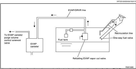
From the beginning of refueling, the air and vapor inside the fuel tank go through refueling EVAP vapor cut valve and EVAP/ORVR line to the EVAP canister. The vapor is absorbed by the EVAP canister and the air is released to the atmosphere.
